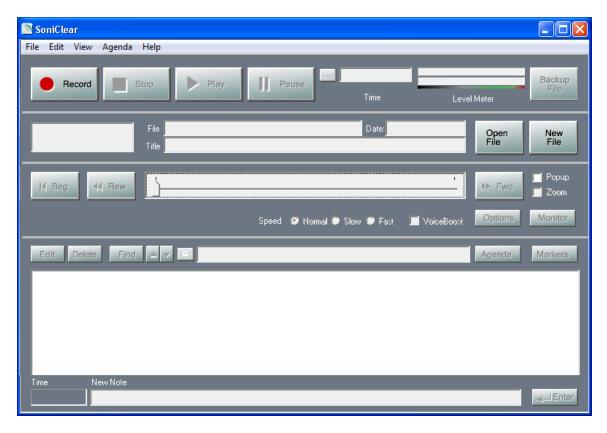
For most applications you can control the program entirely by clicking buttons on the display. On computers with a touch screen, these buttons can also be clicked by touching them. Additional features are accessible from the pulldown menus and the various dialogs that are displayed (see Advanced Features for details).
