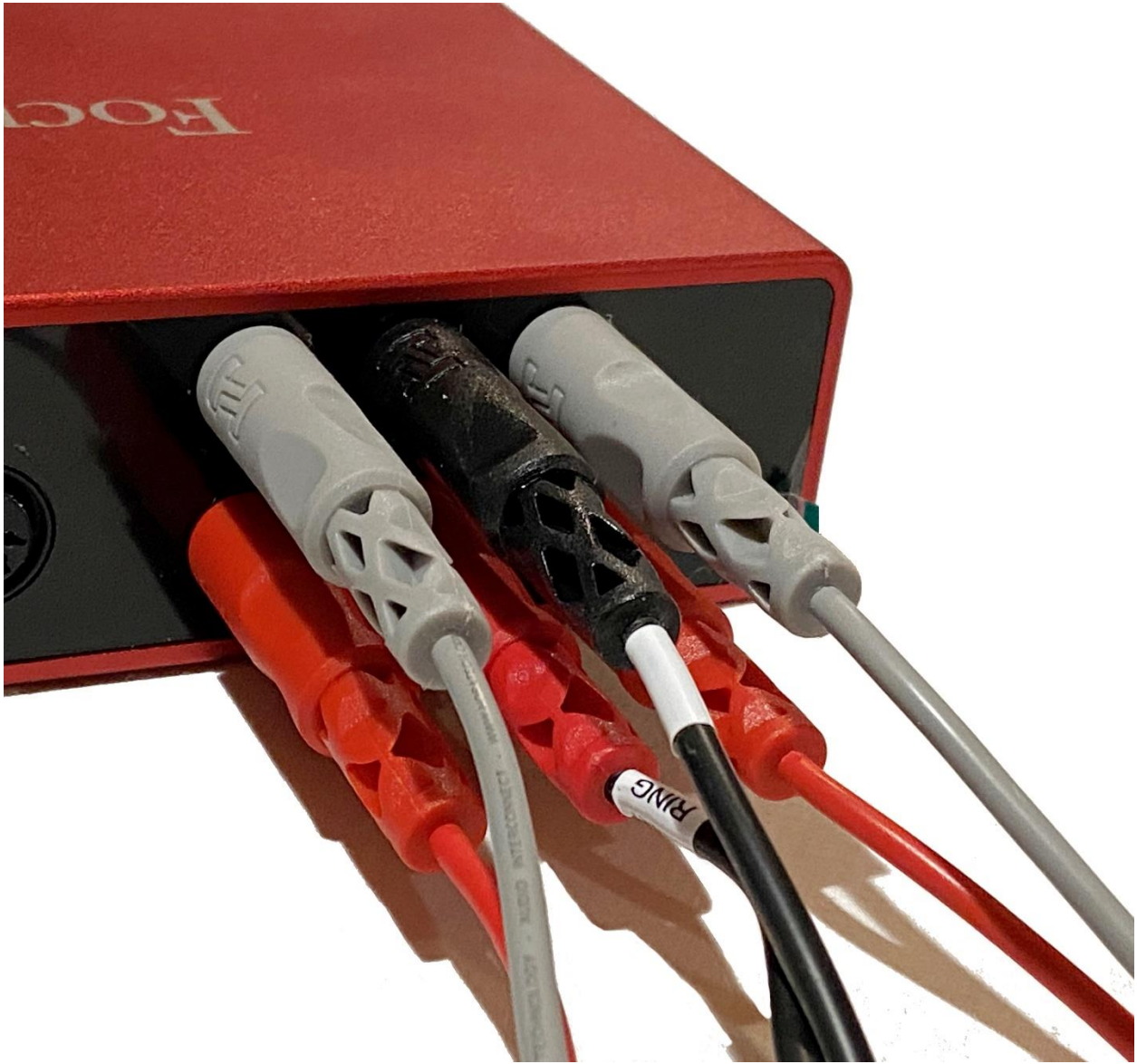
Close up of 1/4" TRS Loopback Cables
