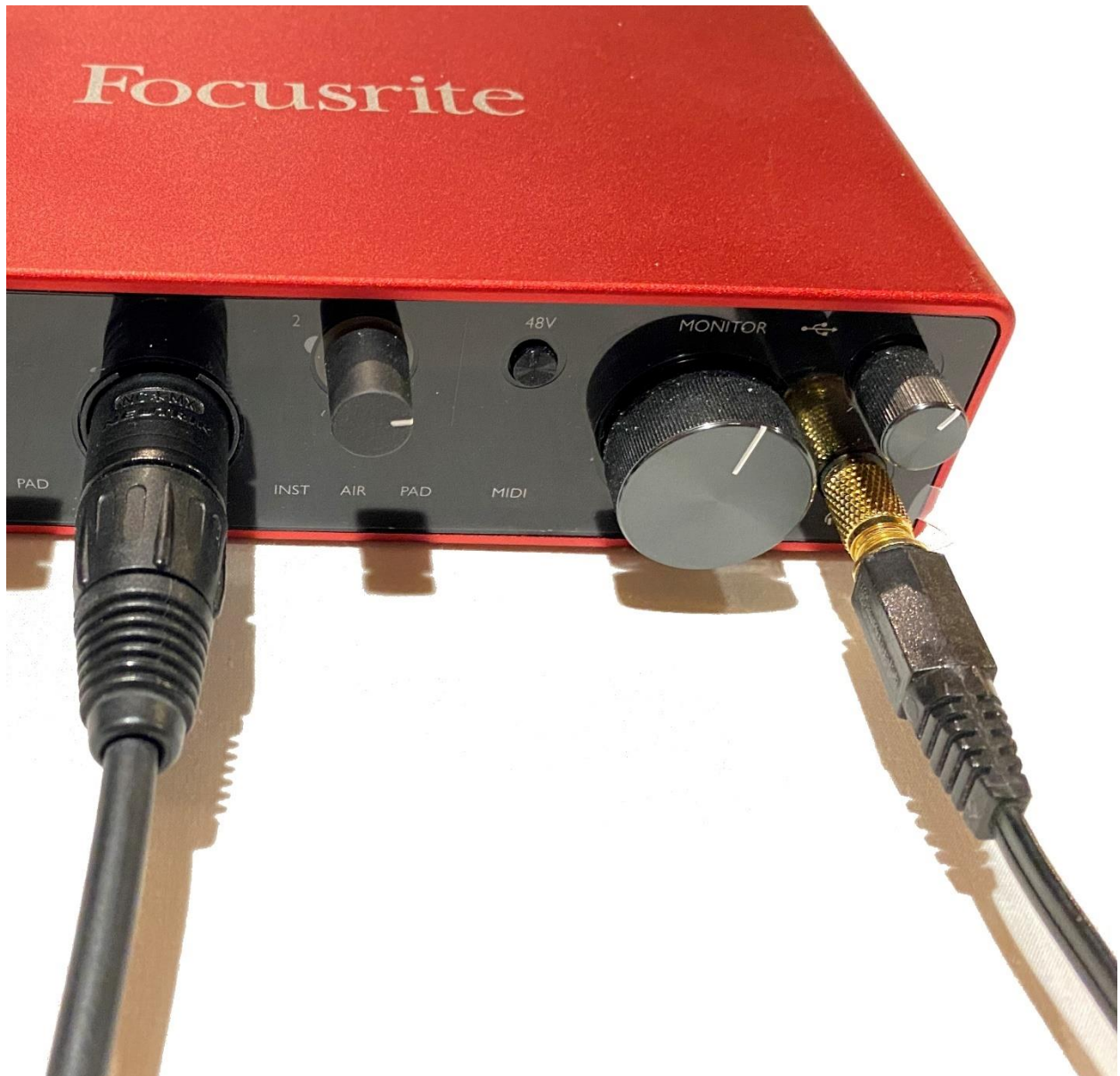
Close up of XLR Microphone and Headphone Connection
